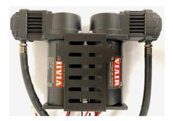
8. Install "Switch Plate" of VIAIR VMS Cradle Bracket: Remove the remaining of original M5 bolts (2) and replace with the provided of 14mm M5 bolts (2) to attach the "Switch Plate".
