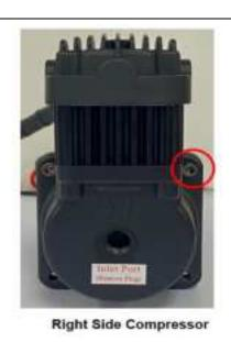
4. Take the compressor for the "Left" side position and slide through the rubber vibration isolator holes. Use (2) 30mm M5 bolts, tighten the bolts to 3-4 ft/lbs., and fasten the (2) bolts using (2) of the provided M5 Nylock nuts and washers.
