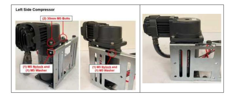
5. Use (2) 18mm M5 bolts and (2) washers to secure the rear of the VIAIR compressor to the Base Plate by sliding the bolts with washers through the rubber vibration isolators.
