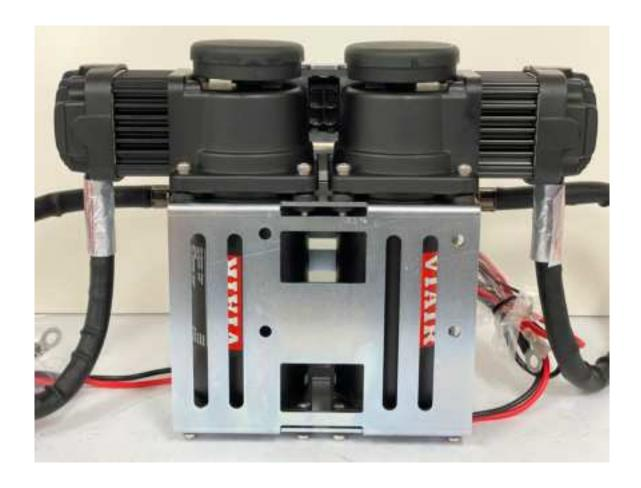
7. Install the "*Top Plate*" of VIAIR VMS Cradle Bracket: Use (2) 14mm M5 bolts on the front-end of VIAIR compressor and (2) 10mm M5 bolts on the rear-end of compressor. *Tighten loosely, do not fully tighten yet.* Once all bolts are in, tighten the bolts to 3-4 ft/lbs.
