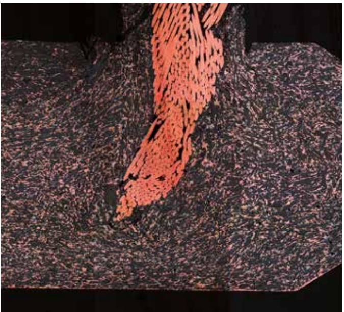
Carbon brush: extensive views of structural homogeneity; distribution of conductive phases such as Cu particles and hard phases; visualization of manufacturing effects
