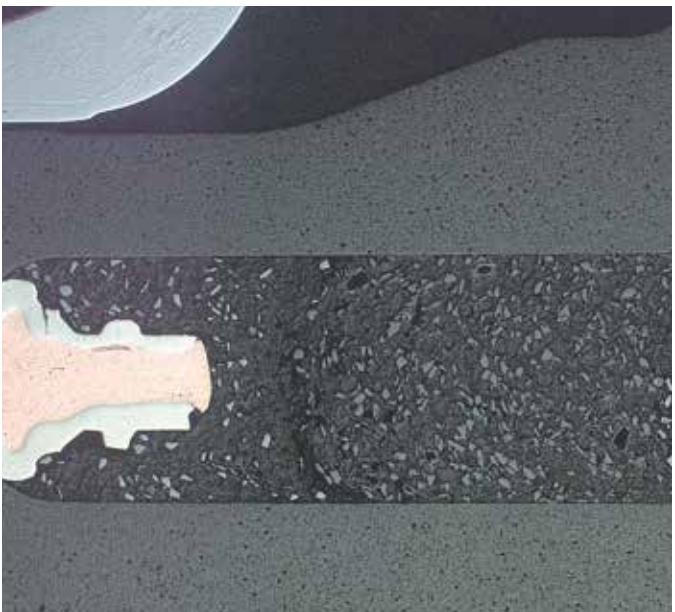
Spark plug: inspection of functional ceramic parts; analysis of different types of material structure such as pore formation in ceramics for insulators, conductive composite materials, and steel and copper pins
