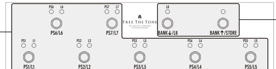
Press this switch in Direct mode to turn on/off LOOP 8 (L8). Note that various functions can be assigned to this switch by the setting done in Edit mode.
