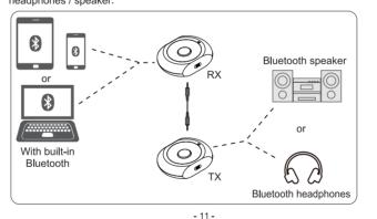
Step 5. Pair your audio source device with the RX unit - Turn on the Bluetooth function on your smart phone / PC, search & select "Avantree Lock" to Step 6. Finish Bluetooth repeater setup - Connect the TX and RX units together using the included 3.5mm-3.5mm connector
