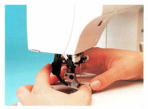
The built-in dual feed/IDT System (Integrated Dual Transport) (Models 6122, 6152, 6232)
