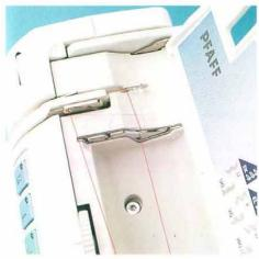
Now, pull the thread into the take-up lever from left to right (19). The take-up lever must be positioned at the very top.
