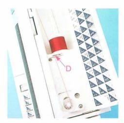
Pass the thread to the right under the guide hook **D**. Then wind the thread several times around the bobbin. Activate the foot control and winding the bobbin with the needle can be started.
