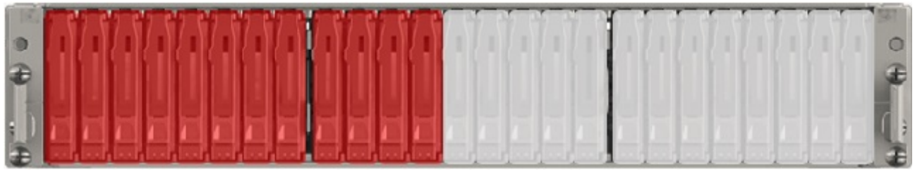
Figure 1. Faulted 25-drive DPE - example
