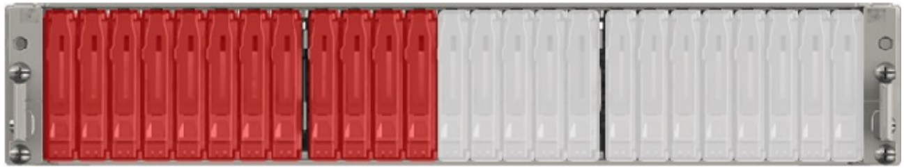
Figure 1. Faulted 25-drive DPE - example
