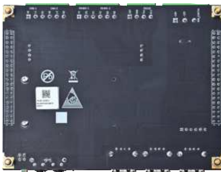
MY-ICEB001 Expansion Board Bottom-view (provided exclusively for MYD-LR3568 with RK3568J version)
