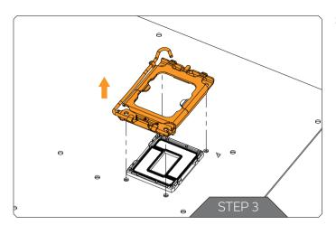
**STEP 3**Remove the stock mounting mechanism from the motherboard.
