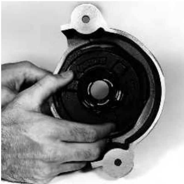
Figure 12 – Remove Jaw Set Cover
