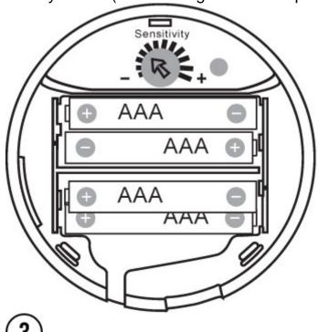
Lock the MultiSensor main unit to it's battery cover by aligning the Lock/Unlock Half-Dimple Markers under the "unlock" symbol and twisting the battery cover from the main unit in a clockwise motion until the Lock/Unlock Half-Dimple Markers form a circle under the "lock" symbol (a
