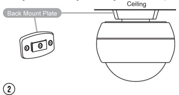
Mounting the Multisensor angled in a direction via the Back-Mount Arm.
