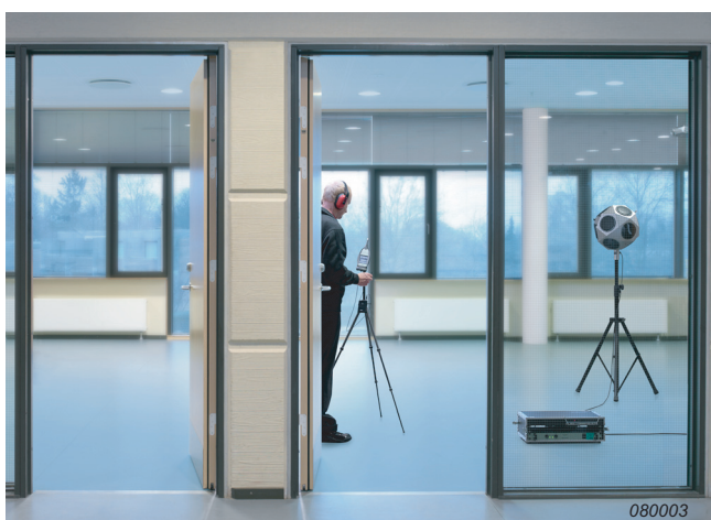
Fig. 7 Reverberation time measurement – measured using the interrupted noise method
