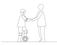
Lightly place one foot on the foot mat, while keeping your other foot on the ground holding your weight. Do not press the steering bar with your leg.
