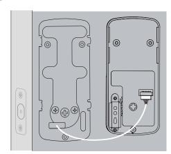
Connect the cable by pushing connector in firmly until it is completely seated.
