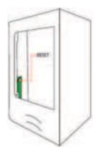
After that date, cylinders should be changed even if they have not been used. It is recommend to return them to your dealer, who will take care of disposal. After removing the screws of the door, is sufficient to remove the cylinder and reset the LED of empty cylinder. After that, insert a new cylinder until you hear the "click" of the plastic support entering in its housing, then close the door.
