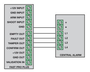
The outputs shown in the diagram are not always necessary, but only in cases where the voltage of pull-up resistance is lower than the power supply one.
