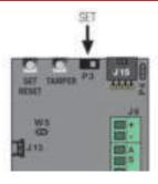
To set the shooting time, after opening the cylinders compartment door, at the top of the PCB, facing the board you must move the jumper P3 in left position (closer to the buttons S1/S2). Holding down the button S1 "SET", 6 leds on the front will flash and each flash is equivalent to one second.
