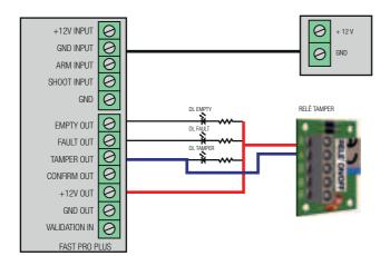
In case of an empty cylinder, the DL EMPTY LED will switch on.
