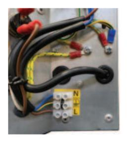
While connecting the machine to the mains power, it is raccomended to never disconnect existing ground cable. The fact of disconnecting or modifing existing cables voids the warranty and can cause troubles or accidents related to the temperature control.
