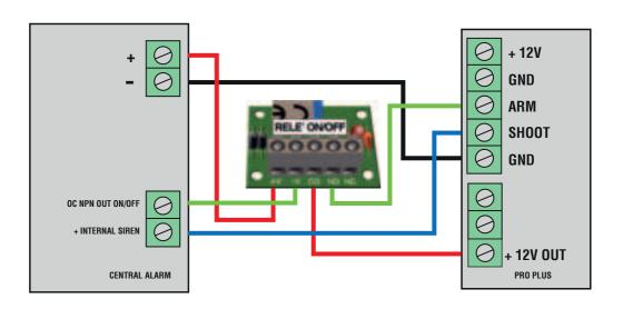
In the diagram above the control panel, as example, provides to UR Fog power supply between 11 and 14V DC 250 mA max. The ON/OFF output of this alarm is an Open Collector NPN opened when the system is off and it is stably closed to negative as long as the system turned on.
