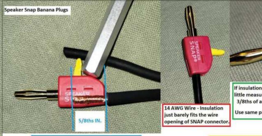
If insulation fits into opening like this 14 AWG wire then use the little measuring gauge built into the connector. Approximately 3/8ths of an inch of insulation will be stripped off in this case.
