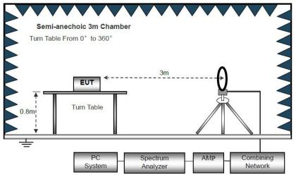
Block Diagram of Radiated Emission Below 30MHz
