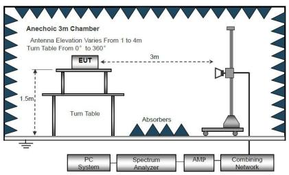
Block Diagram of Radiated Emission Above 1GHz
