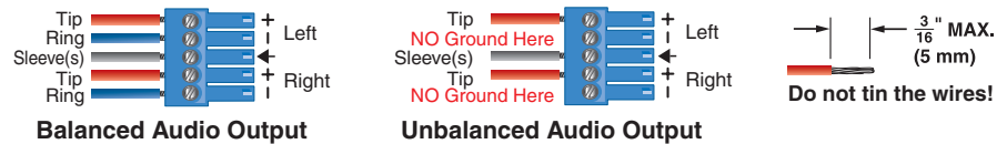
Figure 5. Audio Output Captive Screw Connector Wiring
