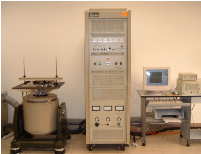
Figure 2.10: Instruments for vibration test
