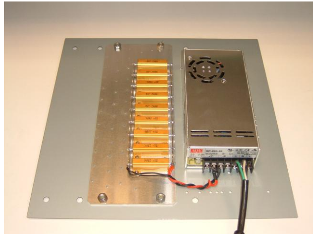
Figure 5.1: Standard setup for EMC test
