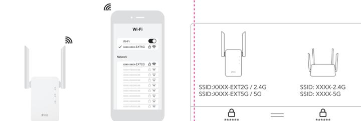
4 Relocate the extender between the Wi-Fi coverage area and the area where you want to expand the Wi-Fi signal.
