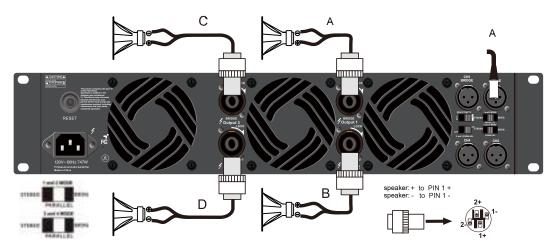
Bridge Connection: Connect the positive speaker wire to the PIN 1+ terminal of the SPEAKON connector, and the negative speaker wire to the PIN 2+ terminal.
