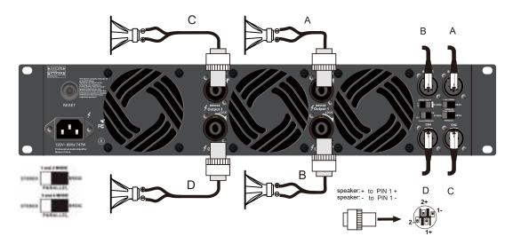
Parallel Connection: Connect the positive speaker wire to the PIN 1+ terminal of the SPEAKON connector, and the negative speaker wire to the PIN 1- terminal.
