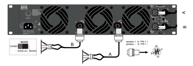
Parallel Connection: Connect the positive speaker wire to the PIN 1+ terminal of the SPEAKON connector, and the negative speaker wire to the PIN 1- terminal.
