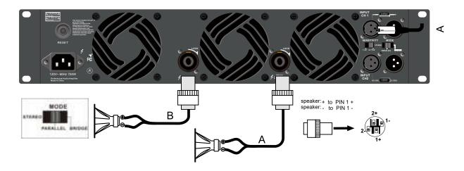
Bridge Connection: Connect the positive speaker wire to the PIN 1+ terminal of the SPEAKON connector, and the negative speaker wire to the PIN 2+ terminal.
