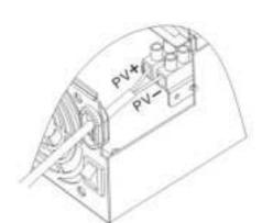
PV+: PV positive PV-: PV negative
