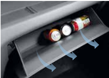
Glove box cooling
