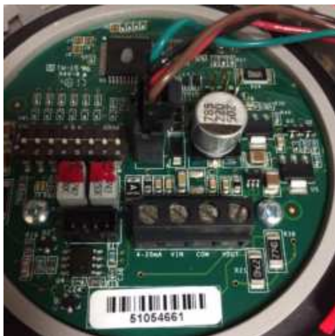
FIGURE 48 8301-067 Sensor Dip Switches
