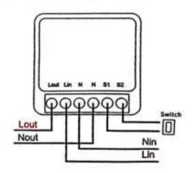
Warning: S1 and S2 can only be connected to the two ends of the wall switch, and cannot be connected to a strong current such as a zero live wire.
