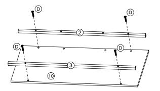
Note: During the assembly, please first half-tighten all the screws into the holes. After all the screws are set, fully tighten them.
