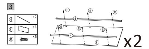
Note: During the assembly, please first half-tighten all the screws into the holes. After all the screws are set, fully tighten them.
