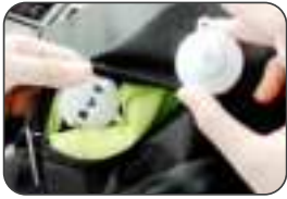
Step 3: Separate the FMN device from the bracket
