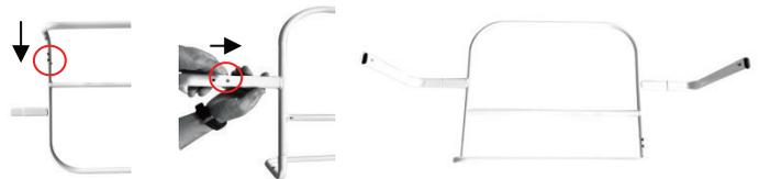
3a) Lay the top frame topside down, and push the middle frame in till you hear a 'click sound'.
