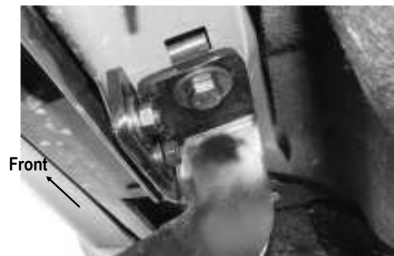
(Fig 4) Passenger Front Mounting Bracket Installation
