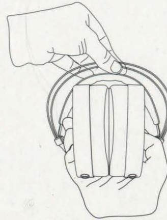
Push down on the headband wire while firmly holding both sides of the headphone with other hand. This will cause the headphone to fold in a controller manner.
