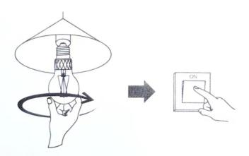
Note: 1. Make sure that the power is off when installing, removing, or examining the light bulb.
