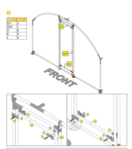
Do not worry too much about the exact location of D3 and D6Y. Just make sure D6Y is completely covered by the two pairs of H.
