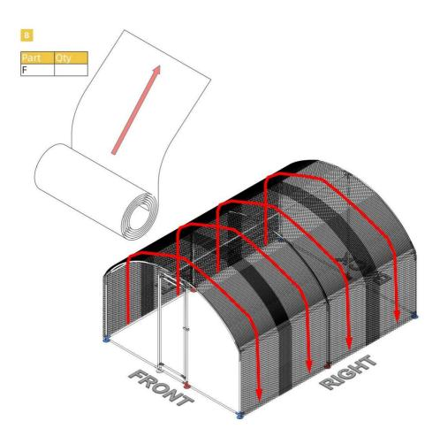
In the package you will find the poultry net. When attaching the net to the chicken run structure, do not precut the net. Instead, roll the net along the tubes and cut it. The arrows on the illustrations indicate the flow of the net. Follow the arrows to roll and cut the net. Use zip-ties to fasten the net to the tubes. There will be overlaps between the nets.
