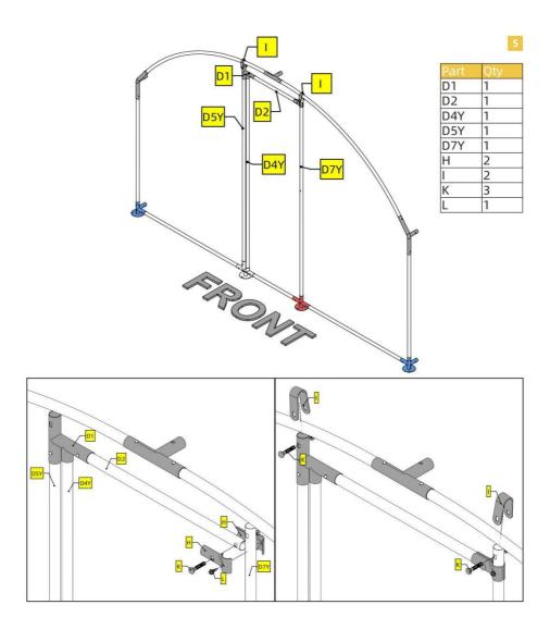
For screw L, you will need a power tool to drive it into tube  ${\sf D7Y}.$
