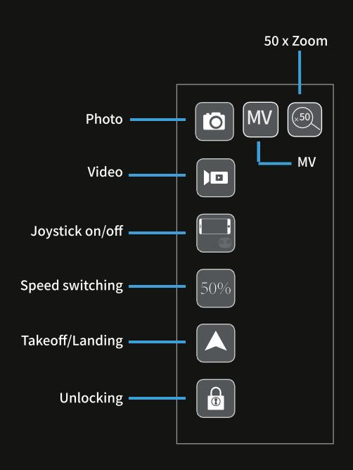
**Photo:** Click the button to take photos according to the current lens (front lens or bottom lens).
