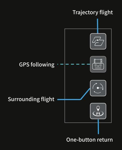
**Trajectory flight:** In GPS mode, the drone will fly according to the location selected on the map.
