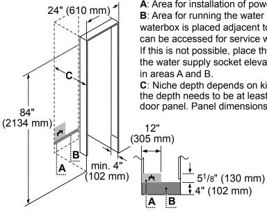
**A**: Area for installation of power connection.
