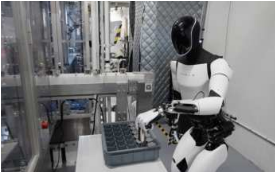
The humanoid robot Optimus features a highly advanced hand with 22 degrees of freedom.
