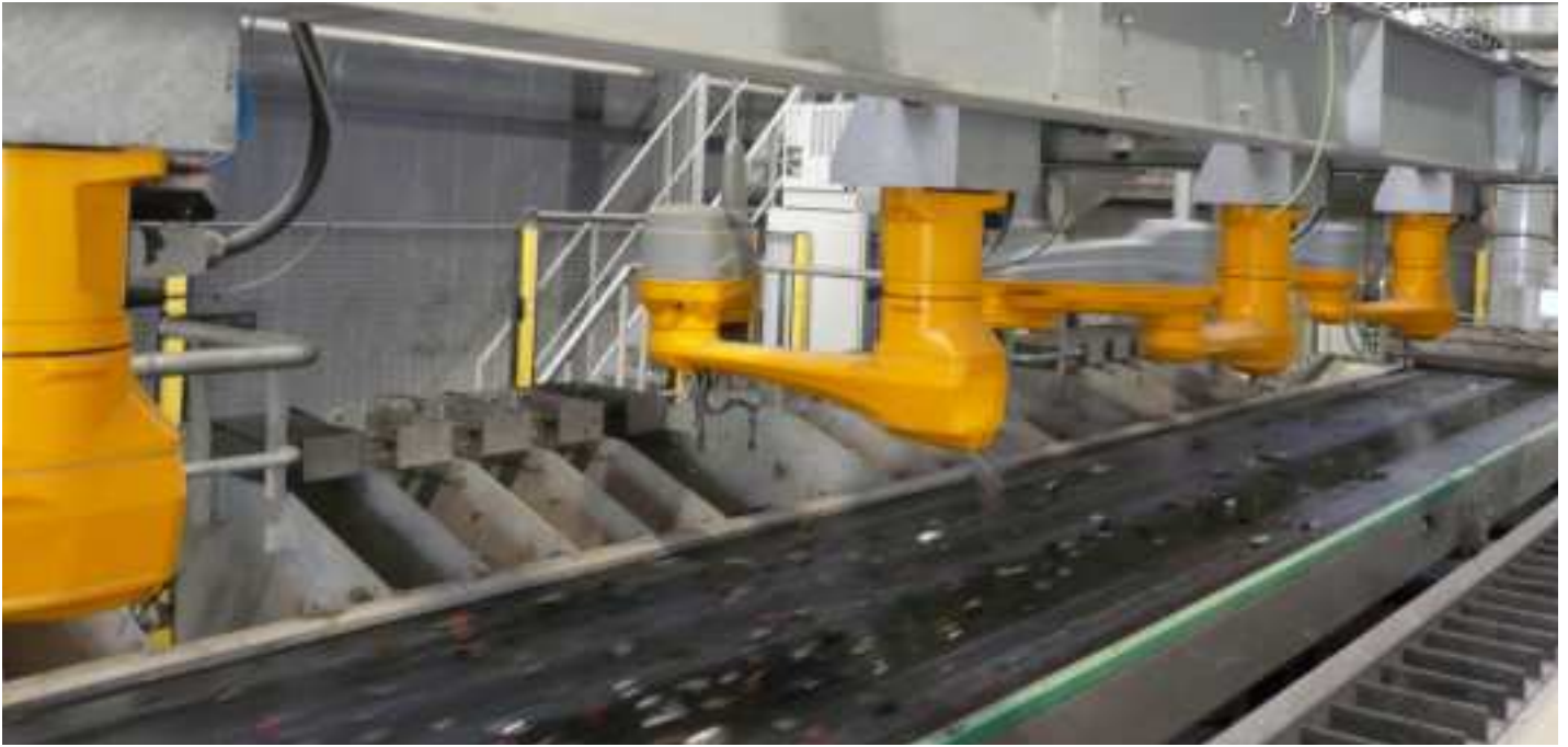
The line is able to sort 15,000 tons of scrap metal per year, with a cycle time of one second per robot.
