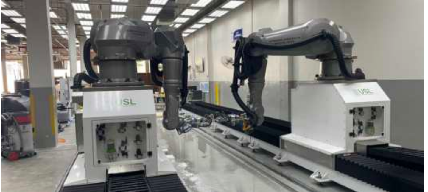
First choice for ultrasonic testing of fuselage components: a duet of Stäubli robots.
