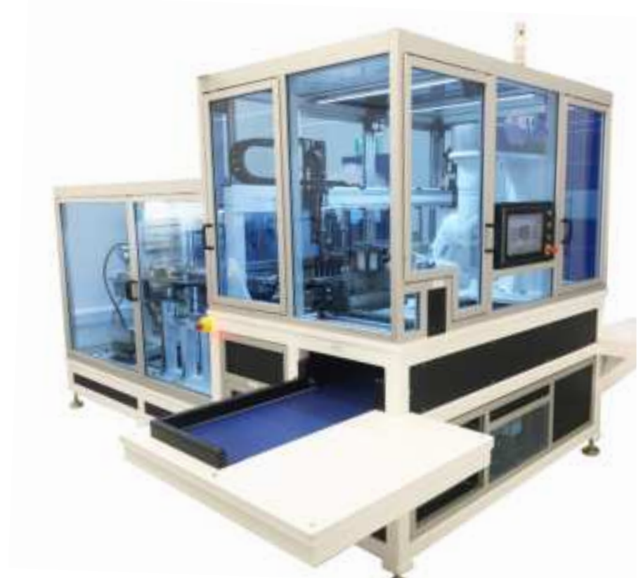
Two Stäubli TX2-60L six-axis robots handle the catheters after inspection with high precision and high hygienic standards.
