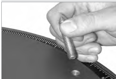
Fig. 49: Remove the pointed bolts from the drive base.
