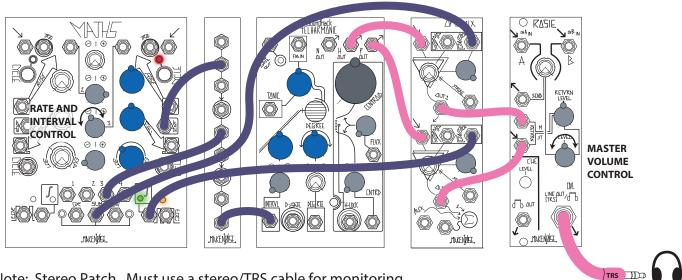
Note: Stereo Patch. Must use a stereo/TRS cable for monitoring.
