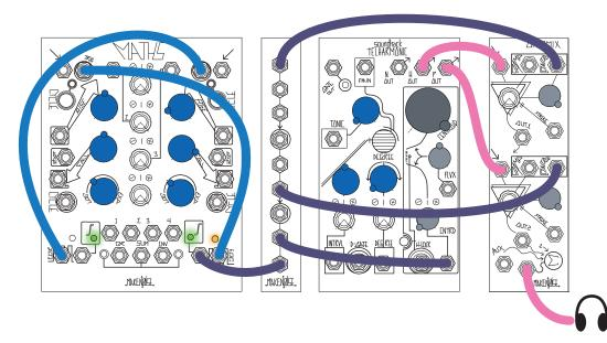
Briefly turn on MATHS Ch. 1 Cycling and wait for Ch. 4 to be triggered via EOR. At which point, press the Ch.1 CYCLE Button again in order to disengage cycling, allowing the trigger loop to continue indefinitely.
