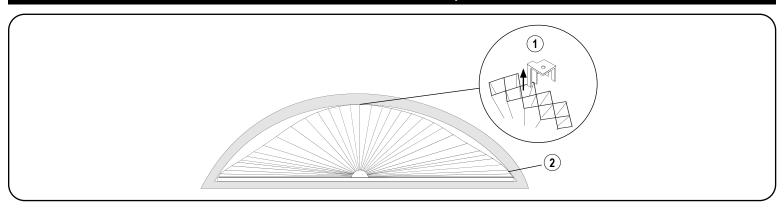
First, find the center of the fabric. Gently press on the fabric until you are able to get the back cell into the top center support clip. Then, go to the first clip up from the bottom of the arch and gently lift and fan out the fabric until the first section fits the window opening. Gently press on the fabric until you are able to get the back cell into the support clip. Repeat for remaining clips. Check the fit of the arch shade. Reposition the fabric in the clips, if necessary.
