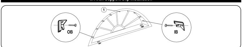
Position the clips so that the back of the clips are the same depth as the back of the installation brackets. First, place a clip at the top center of the window opening and then, space remaining clips evenly apart. Screw the arch support clips to the mounting surface through the hole in the top of the clip (**IB**) or through the slot in the back (**OB**).
