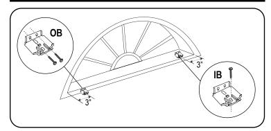
Mount end brackets 3" from each side and space any remaining brackets evenly. Make sure that all brackets are aligned and level.
