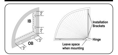
Mount the brackets to the vertical and horizontal mounting surfaces. Place brackets approximately 3" from the bottom and the top along the vertical mounting surface. Then, place a bracket approximately 3" in from both edges of the horizontal mounting surface.
