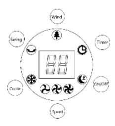
Insert the plug into the electrical outlet. Press the "On/Off" button to turn the unit "ON". The LED indicator automatically shows the room temperature and shifts the fan to standby mode. The functions of the unit can be controlled via control panel or by remote.
