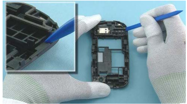
30) Use the SS-93 to release the MAIN ANTENNA.
