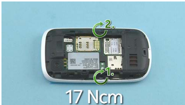
9) Tighten the two Torx+ size 6 screws to the torque of 17 Ncm.
