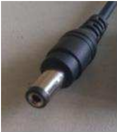
DC male connector :5.5x2.1mm
