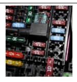
Note: Install the fuse adaptor in the fuse box (Cavity No. F41) as shown.
