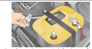
Note: Connect the -ve terminal of car battery after the installation.
