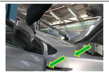
Note: Route the harness using the flexible steel wire in the arrow direction from step 30 31 to 33.
