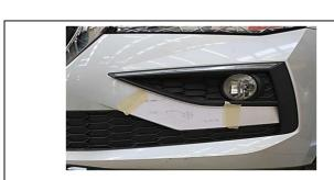
Note: Stick the template and cut out region where the brackets will be installed using the drill bit provided with the kit. See step 3-11.
