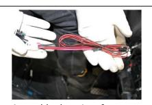
Note: Assemble the wires from sensor harness to the 16-pin white ECU connector available in the power harness. Follow step 47-50 for all the pins.
