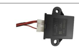
Note: Assemble the Power harness connector into the ECU.
