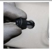
60 Note: Install the switch into the dashboard.
