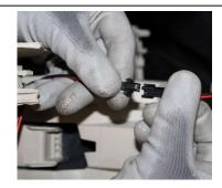
Note: Connect the switch wire with the power harness as shown.
