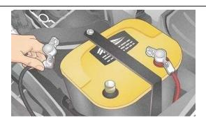
Note: Ensure -ve terminal of car battery is 1 disconnected before starting installation.
