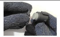
Detach the rubber ring available on sensor head and keep it aside as it need to reattach after 1 completing the painting process.
