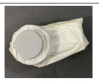
Mask the whole sensor except the head using  $^{4}$  the masking tape  $\ .$
