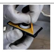
Note: Peel off the adhesive protection layer 19 from the tape.
