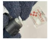
Remove the dust from the sensor by cleaning 3 the surface with SWAB or alcohol dipped cloth.
