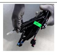
Note: Attach the sensor harness connectors 22 to all the four sensors.
