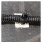
Note: Route the harness and tie with the cable ties, after tightening cut the extra edge 28 of cable ties.
