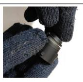
Re-attach the rubber ring back on the sensor head.
