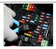
Note: Pull out the 7.5A fuse (Cavity No. F41) from the fuse box.
