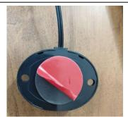
Note: Peel off the protection layer of DSA tape.
