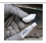
Note: Now apply the Primer around the hole 17 using the cotton and wait until its dry.
