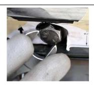
11 Note: Tighten the screw until hole is formed.
