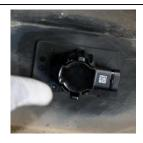
Note: Paste the bracket at designated location as shown and bracket should be pasted with the sensor in assembled form to avoid sensor position mismatch.
