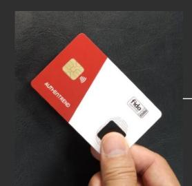
Take the card by "enrolled" thumb finger (on fingerprint sensor sear) and index finger (on back)
