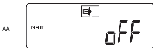
The UPS is locked
