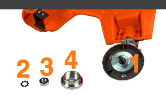
Remove the floating disc (2) and washer (4).Place the mounting disc (1) on the shaft.
