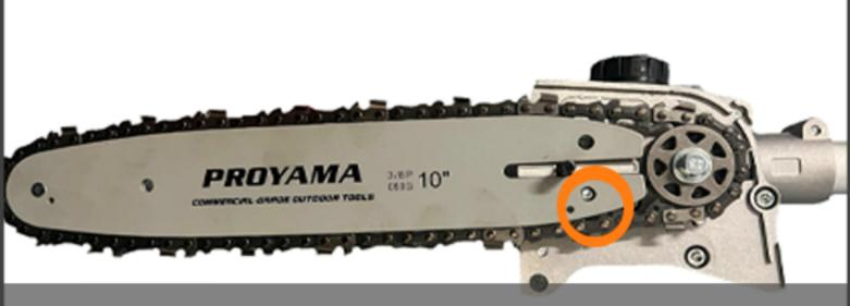
Loop the saw chain around the drive sprocket and install the guide bar onto the bar-retaining studs.
