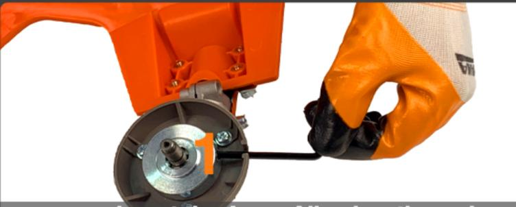
Insert the 4 mm Allen key through the winding guard and the mounting disc (1) into the opening on the angle gear (blocks the angle gear). Necessary turn the mounting disc (1) slightly.
