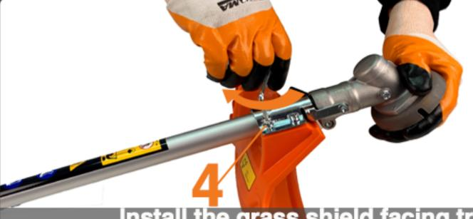
Install the grass shield facing trimmer head by placing (4)bolts through the plate grass shield assembly and fasten the bolts to the grass shield clockwise using the larger sized (4mm) Allen wrench provided.
