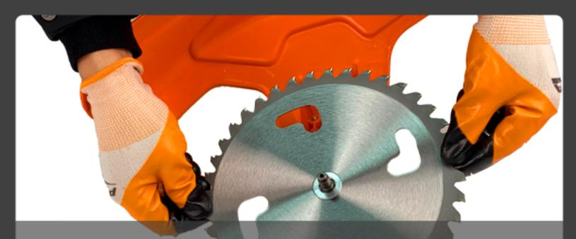
Position the blade 40 teeth Blades must be installed like fig8( teeth toward direction of rotation)
