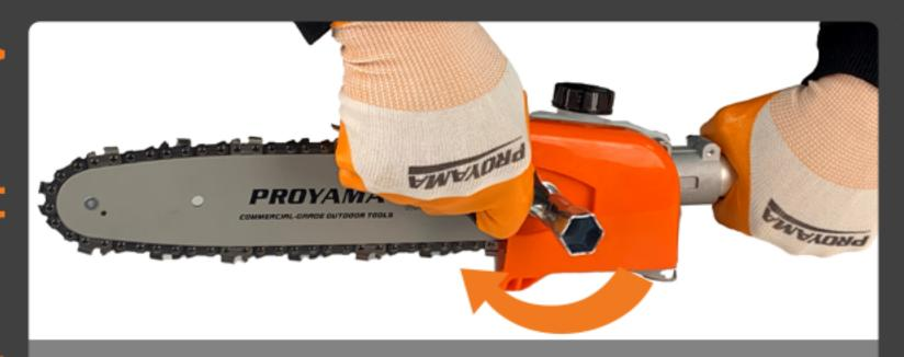
Tighten the bar nuts with the combination wrench.
