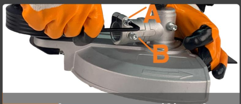
Loosen screws (A) and remove locator screw (B) on hedge trimmer cutting attachment.
