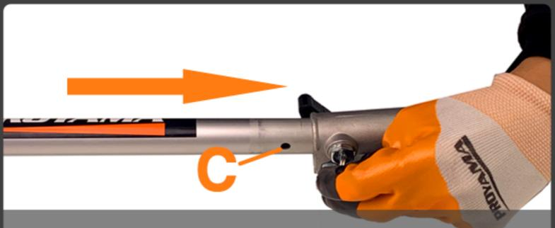
Pull out the locking pin, Insert the pole saw attachment shaft, lining up the locking hole with the locking pin.
