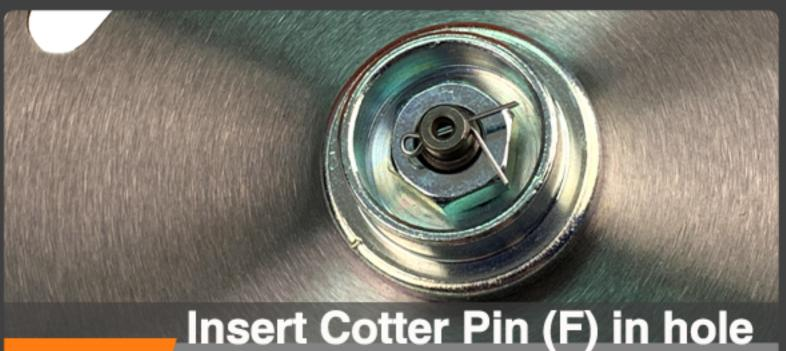
in shaft, and bend pin legs around shaft counter clockwise to retain 10 mm nut.
