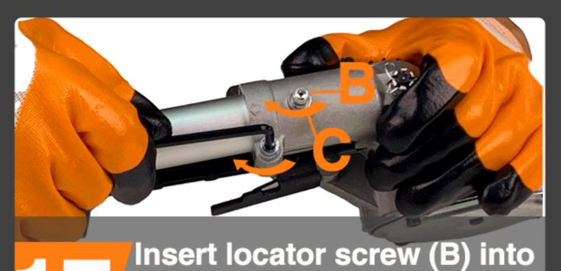
hole (C) and tighten to snug.
