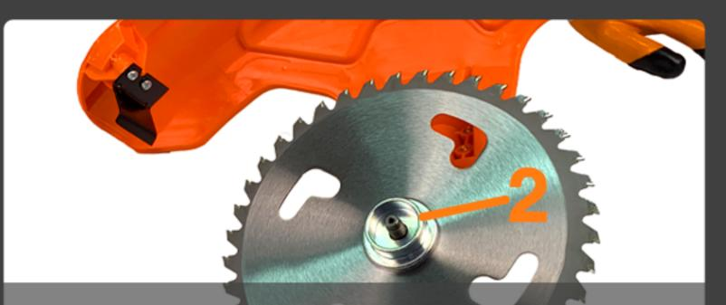
Set the floating disc(2) onto the blade or circular saw
