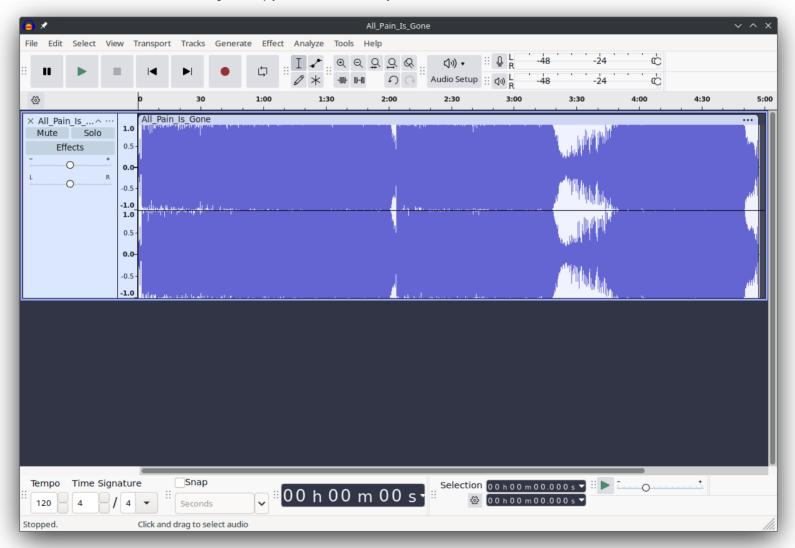
Pres Ctrl Key + A to select all audio track and than click on: Effect  $\rightarrow$  EQ and Filters  $\rightarrow$  Low-pass Filter
