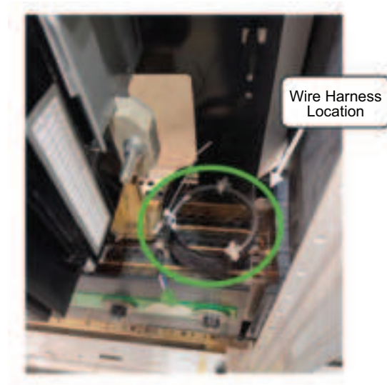
Figure 2 - Shipping Location of Pre-Assembled Wire Harness
