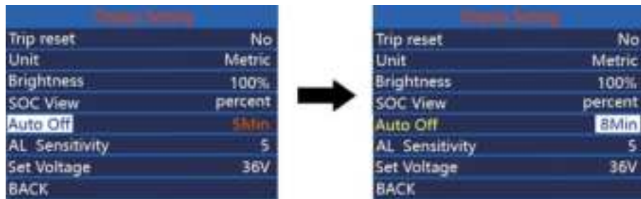
Automatic shutdown time setting interface
