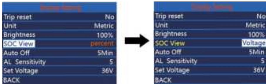
Battery percentage/voltage display setting interface
