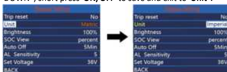
Imperial and metric unit conversion setting interface
