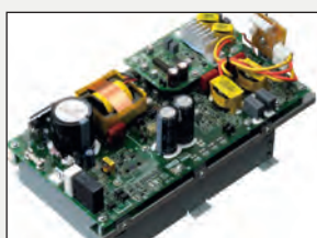
HIGH-EFFICIENCY 1100W CLASS-D AMPLIFIERS
