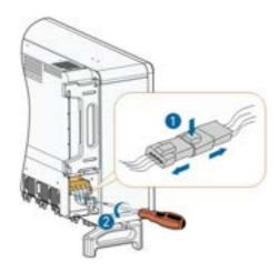
step 4 Pull out the fan module, clean the fans with soft brush or vacuum cleaner, and replace them when necessary.
