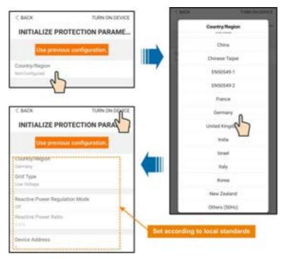
figure 7-4 Initialization Protection Parameter
