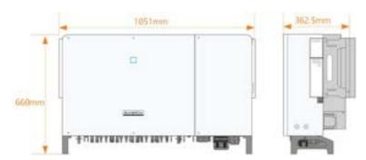
figure 2-3 Dimensions of the Inverter(in mm)
